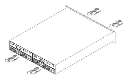
Figure 8. Airflow through the storage subsystem
